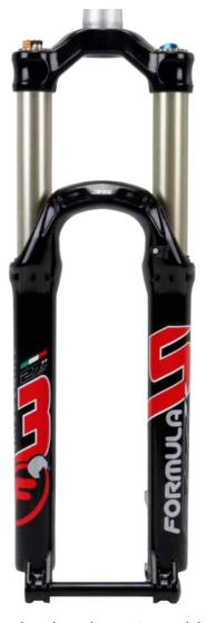
Formula makes a shorter piston rod that's designed for a different fork. Fitting one to the Thirty Five would enlarge the air chamber, making the spring more linear and able to use all of its travel. You could consider this custom modification if you have similar problems with utilising full travel.
